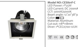
Model NO: CES801F-C LED Power: 1\*25W LED Current: DC 700mA\*1 CCT: 3000K/4000K Beam angle: 12°20°38°50° Color: Material: Aluminum Cut-out: 118\*118mm
